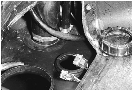
Large opening to left is for fuel pump, smaller for sender. Screw cap shown at right. Hoses in background are for filler and vent. The near connector is for the fuel pump, the 3-wire is for sender.
