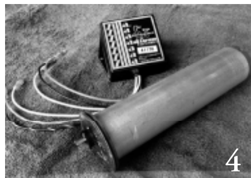
Tankzilla sender and electronics box. Old connector is crimped to the red, black and white
