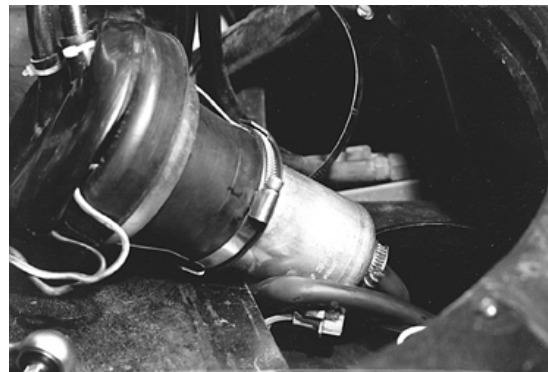
Fuel pump about to be installed. Fuel supply nose on bottom of pump. Return hose on side. Note how hose clamp end is captured in the support ring.
