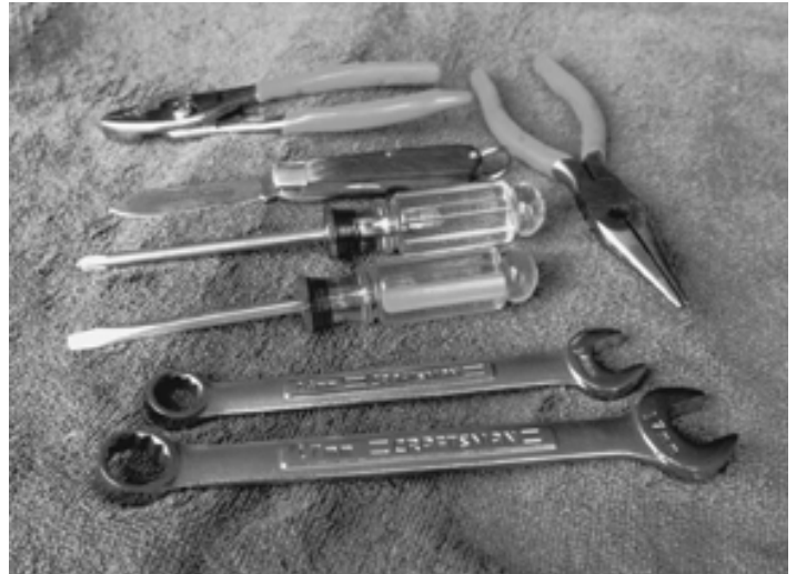
All the tools necessary to repair fuel pump and related items. Handy, but not necessary: diagonal cutters and small 1/4" ratchet.
