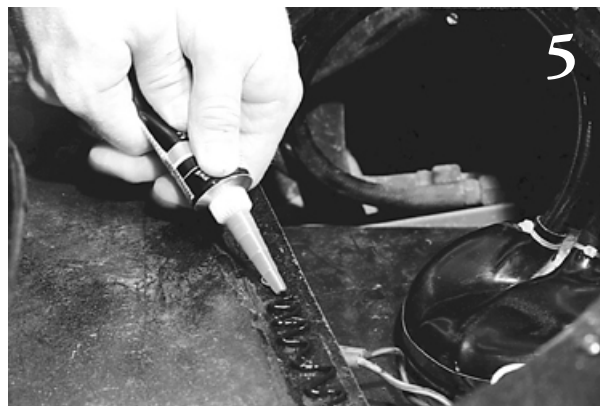
Applying black silicone RTV. Be generous.
