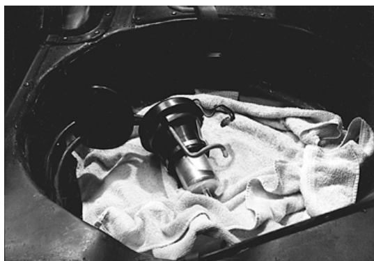
Fuel pump with new sealing ring installed.
