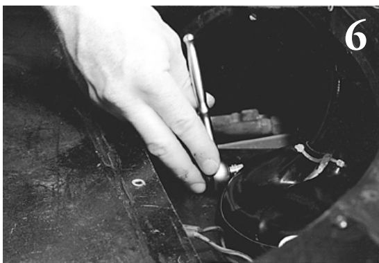
Tightening (or removing) the hose clip around the cover seal/sealing ring.
