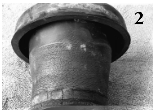
Bad fuel pump sealing ring - note severe checking in rubber.
