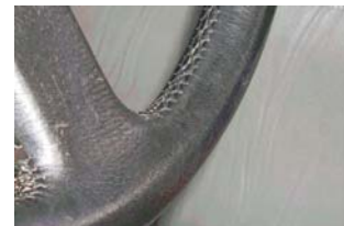
Figure 17 Correct stitching, steering wheel
