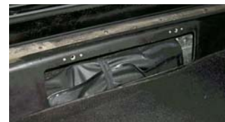
Figure 23 Properly stowed jack
