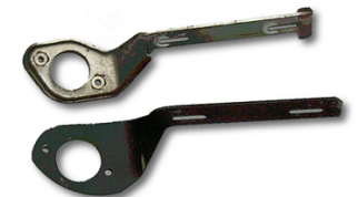
Figure 40 Incorrect bracket bottom
